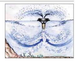
After one month in operation, dissolved oxygen (D.O.) readings were taken again at each of the three sample points listed above. At each location in the water column, it was realized that D.O. levels had risen 2mg/I. The increase in levels at the deeper depth demonstrates that the aerator draws the deeper water up through the pumping chamber.
