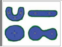
Placement of an aerator can vary depending on the pond condition and shape. A single aerator should be placed in the area that will give you the greatest amount of circulation. If the pond has severe algae conditions or is irregularly shaped, more than one aerator may be best to generate the maximum circulation. When sizing a system for aeration Otterbine recommends 2HP per surface acre.
