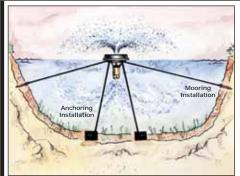
Otterbine aerating fountains, surface spray industrial aerators and fountain units are typically moored from shore to shore or anchored to the bottom of the pond as depicted in the illustration. The power control center is mounted on shore and then insulated underwater cable is run from the power control center to the unit. For more information on installation, please visit our website at www.otterbine.com.
