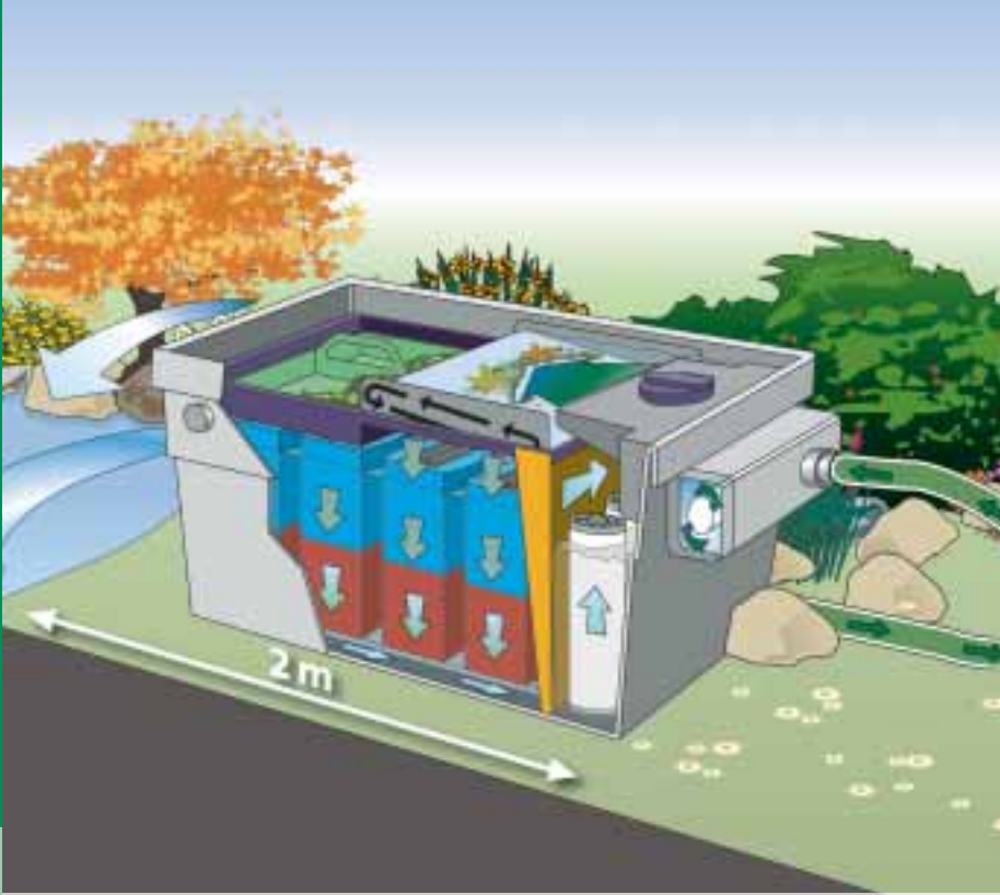
Schematic diagram: UVC in combination with OASE BioTec ScreenMatic
