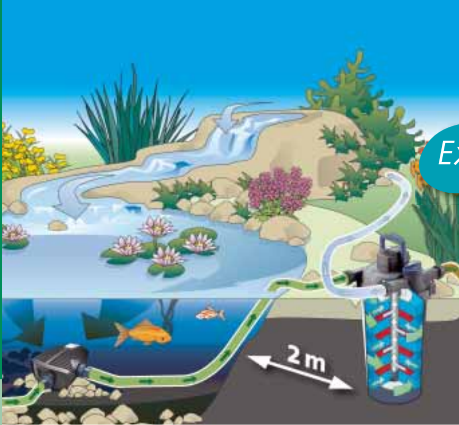
Schematic diagram: Pressure filter FiltroClear in combination with filter and watercourse pump
